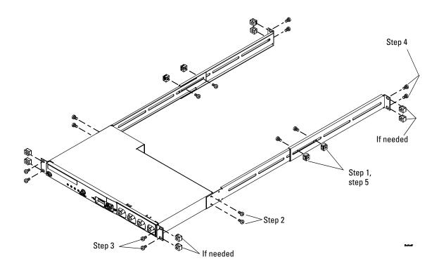
1 Loosely attach the Front Extender Supports to the Rear Extender Supports with four (4) clip-nuts and four (4) of the 10-32 x 0.375 Rail Screws. (The screws require a Torx T20 driver.) Choose the correct set of slots in the supports such that their overall length is approximately correct for the depth of your cabinet.
